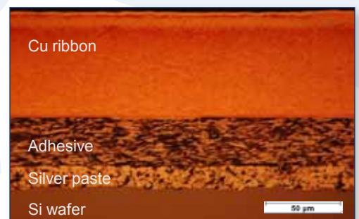
Polished cut section of contact on c-Si
