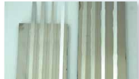
Peel test sample on thin film substrate
