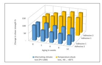
Thermal conductivity (left) and shear strength (right) of adhesives vs. various aging conditions
