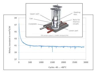
Thermal resistivity of gap filler vs. thickness (left) and vs. no. of power cycles (right)
